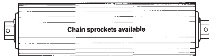
3 1/2" DIA. — 1090# CAP. 5850# with precision bearings
