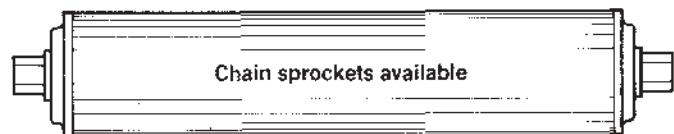
2 1/8" DIA. — 580# CAP. 3350# with precision bearings
