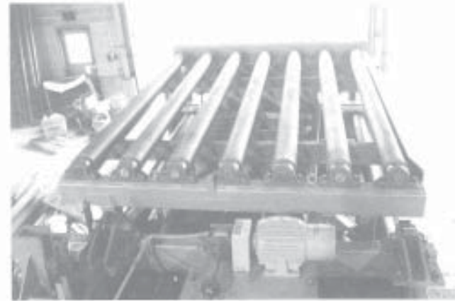
These large diameter heavy-duty chain driven rollers are mounted on pillow block bearings. This is part of a system to handle 20,000 # stacks of steel blankings. The conveyor will interface with AGV's (Automatic Guided Vehicles) at receiving.
