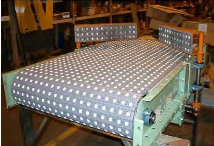
This special plastic belting has roller built into the belt. Allows easy diversion of product to other conveyors. Center device shown centers load.
