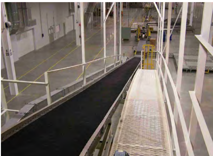
Belt Conveyors are used extensively for moving product to different elevations. This moves appliances from assembly to shipping.
