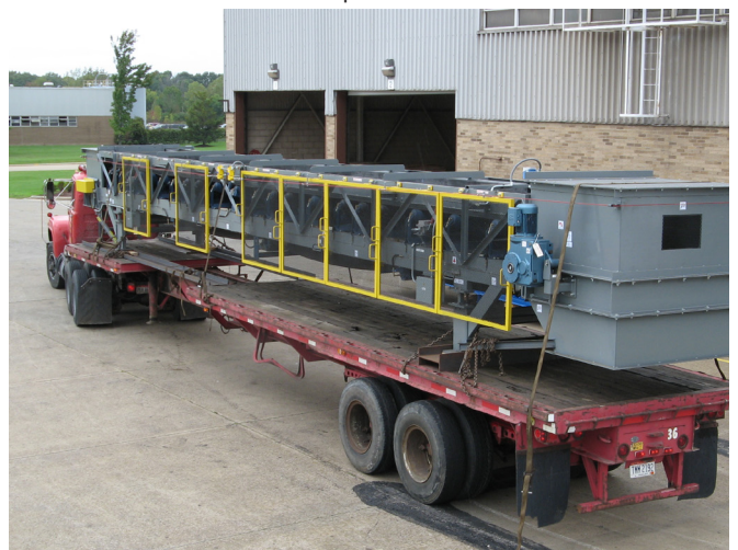
Foundry troughing conveyor for feeding furnaces. Has built in weigh scales for material input.
