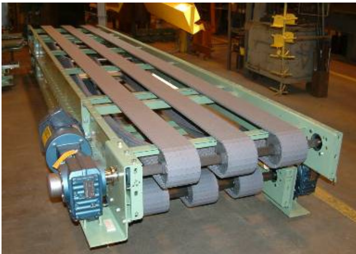
This belt conveyor features plastic belting.
