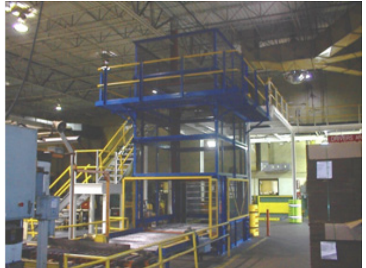
WEBB-STILES continuous Speedlifts from 100 to over 3000 pound load capabilities are a must where production and high cycle times are called for.
